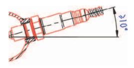
Recommended design of the mating thread in the exhaust pipe \*: THexagon > 600°C or TGas > 930°C
